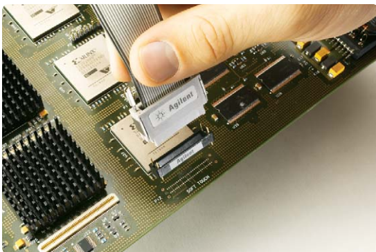
Figure 22. Designed-in soft touch connectorless probe
